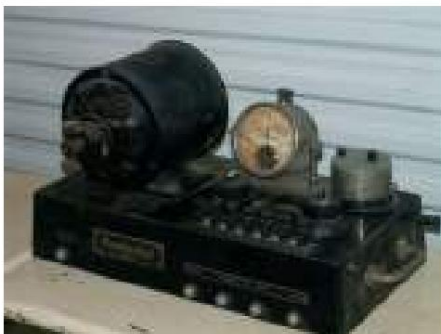
Photo 6. The Pantostat was used by physicians in physical engineering for Galvanization, Electrolysis and Iontophoresis in the early 1900's
